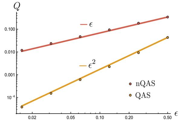
**Fig. 2.** Test of QAS at first order in size of non-axisymmetric perturbation; note the measure
