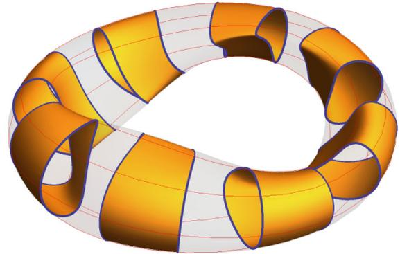
**Fig. 1:** Flux surface shape induced by quasiasymmetry-preserving perturbation (assuming circular zeroth-order shape).
