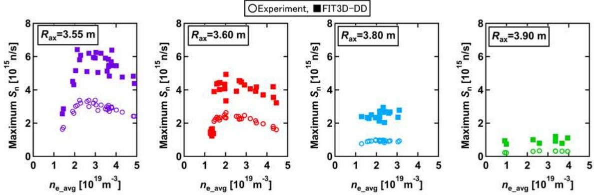
**Fig. 1.** Electron density dependence of total neutron emission rate  $S_n$  for  $R_{ax}$  from 3.55 m to 3.90 m.
