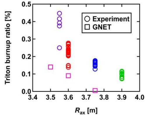
**Fig. 5.** Triton burnup ratio dependence on  $R_{ax}$  obtained in experiment and GNET simulation.
