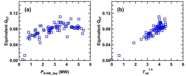
**Fig. 2.** Dependence of equivalent  $Q_{DT}$  on (a) NB deposition power and (b)  $T_{e0}^{1.5}$ . Equivalent  $Q_{DT}$  reached 0.11.
