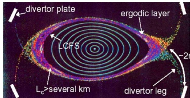
Fig. 1. Poincaré plot showing the LHD flux surfaces, ergodic layer, and divertor legs. Source: Y. Feng et al., Nucl. Fusion 49 (2009) 095002.
