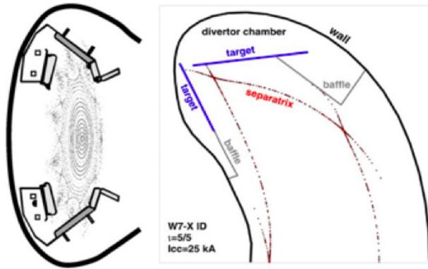
**Fig. 2.** Poincaré plots of the Wendelstein 7-X line of island divertors. Source: IPP-Greifswald.
