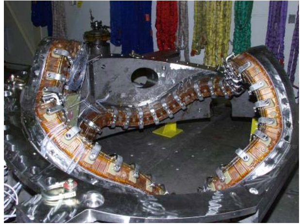
Fig. 1. Completed modular coil.
