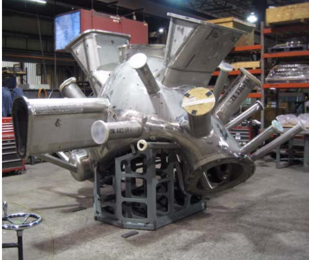
Fig. 2. Vacuum vessel segment with ports attached for testing.
