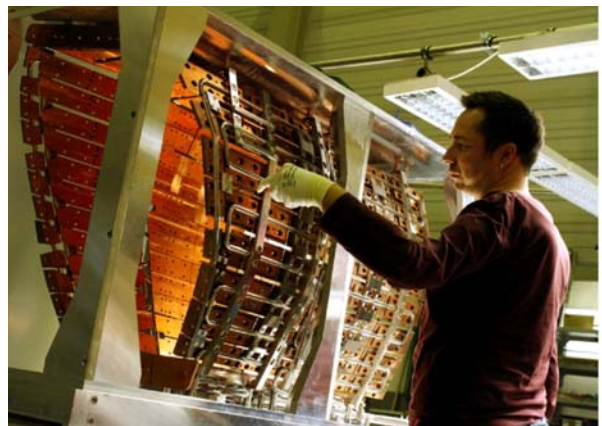
Fig. 3. Wall protection prepared for a port to be used for neutral particle heating. Photo: IPP, Robert Haas
