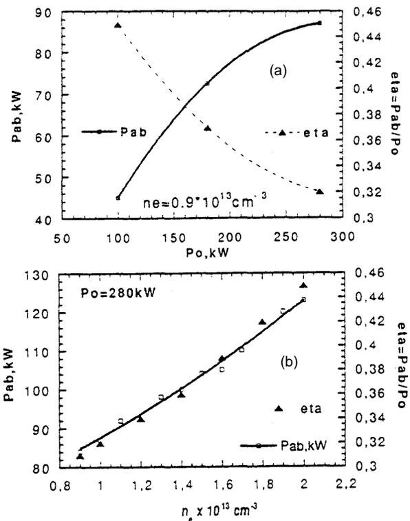
Fig. 1.  $W$  and  $\eta$  ( $\eta$ ) dependencies on (a) input heating power and (b) plasma density.
