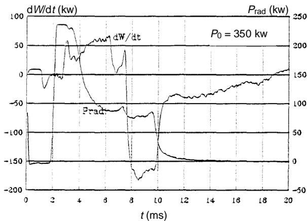
**Fig. 5.** Time behavior of  $dW/dt$  and  $P_{\text{rad}}$  for a quasiradiation type of an ECRH discharge.
