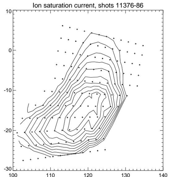
Fig. 1. Bean-shaped density profile in H-1 obtained using new 24-tip Langmuir probe. Data from 11 channels are shown.
