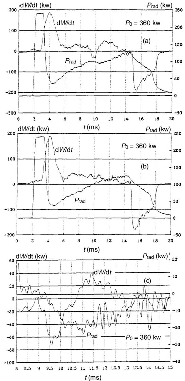
**Fig. 3.** Time behavior of  $dW/dt$  and  $P_{rad}$ , (a) with ECRH power modulation; (b) without modulation; (c) the effect of the power modulation on  $\Delta(dW/dt)$  and  $\Delta(P_{rad})$ .
