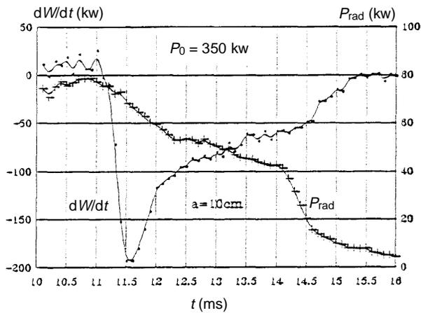
**Fig. 4.** Time behavior of  $W$ ,  $dW/dt$  and  $P_{\text{rad}}$  for two-step plasma decay.
