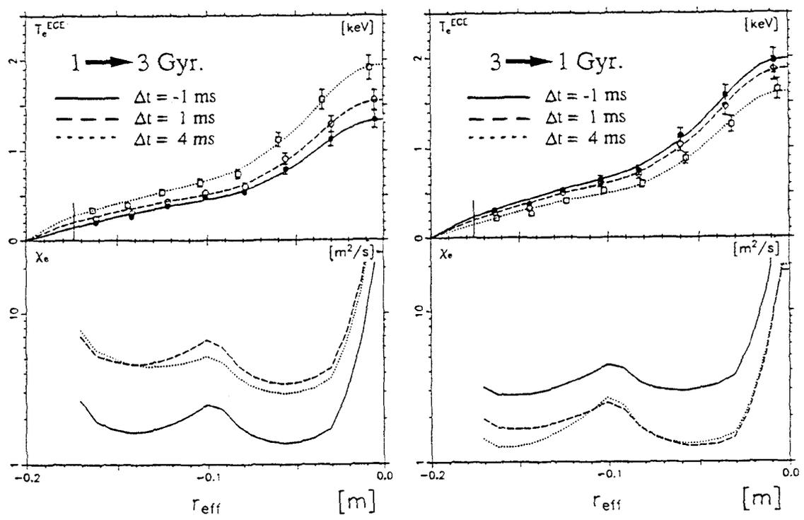
Fig. 2.  $T_e$  and transport coefficient profiles before and after (1 and 4 ms) the gyrotrons are switched on (left) and switched off (right).
