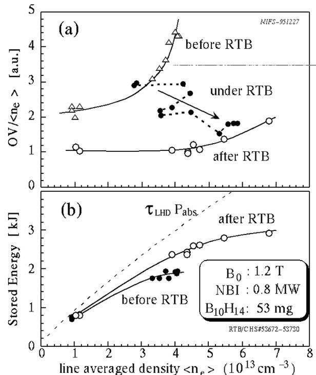
Fig 2. (a) The O V intensity and (b) the plasma stored energy (the broken line represents the quantity calculated with LHD scaling).
