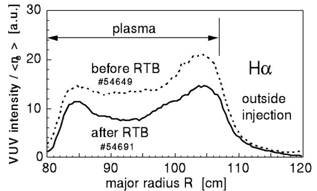
**Fig. 4.** The poloidal distributions of the  $H_\alpha$  intensity before and after RTB with outside (125-mm) injection.
