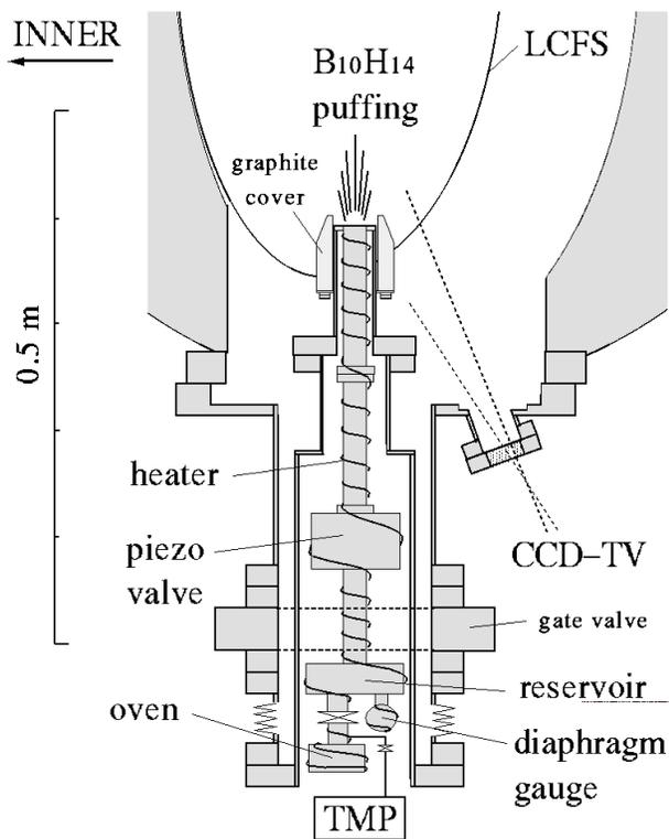
Fig. 1. The movable gas-puffing RTB device in CHS.
