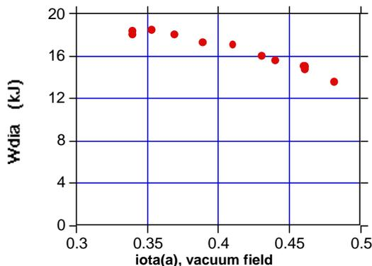
**Fig. 5.** The diamagnetic energy content of discharges 31900–31912 and 31914 for maximum NB heating power as a function of the vacuum field rotational transform  $\iota$  at the plasma boundary. A maximum value of  $W_{dia} = 18.5$  kJ is seen in discharge 31911 at  $\iota = 0.353$ . The discharge conditions in this series are similar to those in Fig. 2 ( $\iota = 0.38$ ), except for the smaller vertical field of about 200 G. (R. Jaenicke)
