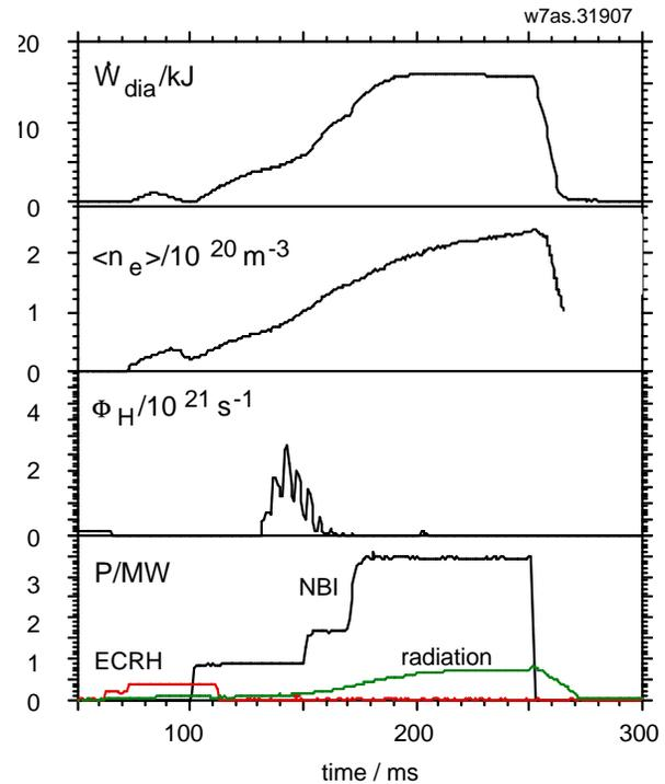
**Fig. 1.** Development of discharge 31907. From top to bottom: Diamagnetic energy, line-averaged density, external gas flux, and ECRH and NBI power input and bolometer radiation signals, respectively. (Courtesy R. Brakel)
