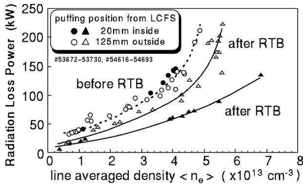
**Fig. 3.** Comparison of RTB effectiveness with injections from 20 mm inside and 125 mm outside the LCFS, where the total mass of decaborane used was 53 mg in both cases.
