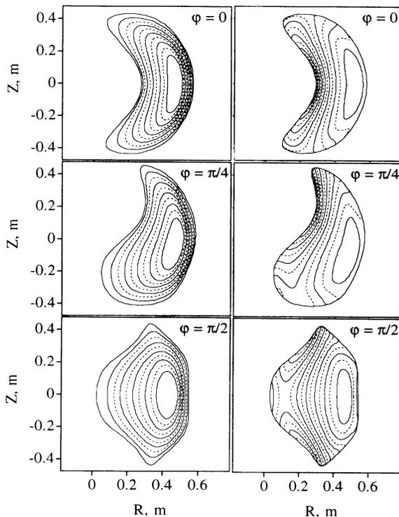
**Fig. 6.** High- $\beta$  ( $\beta_0 = 86\%$ ,  $\beta = 20\%$ ) MHD equilibrium in the DHS with self-consistent bootstrap current. Left: flux surfaces. Right: contours of  $|B|$ .
