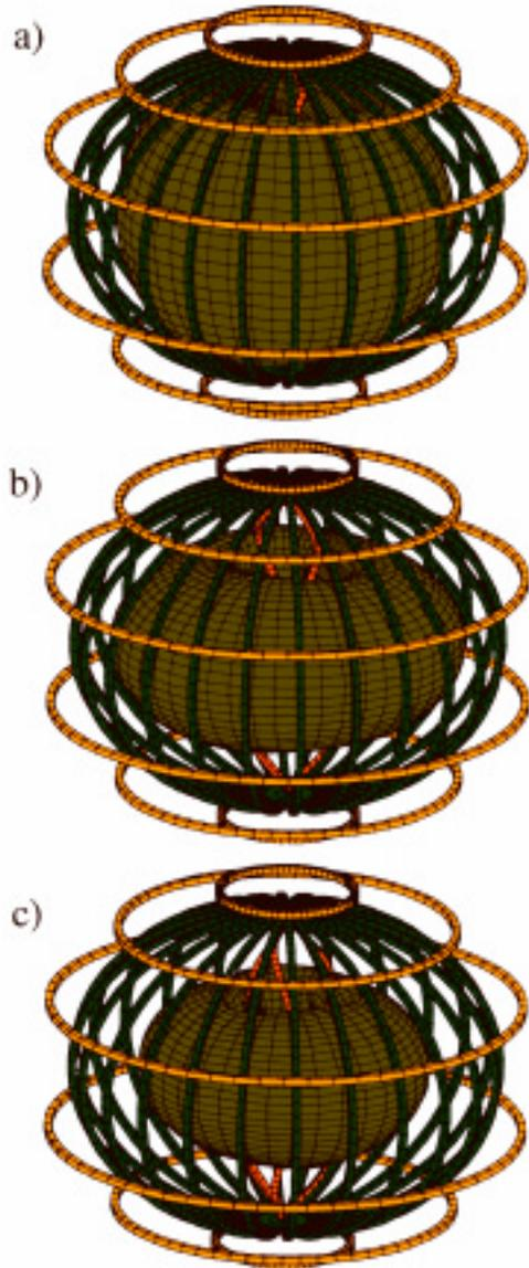
**Fig. 1.** The coil systems and LCFS of (a) SHS, (b) DHS, and (c) THS.
