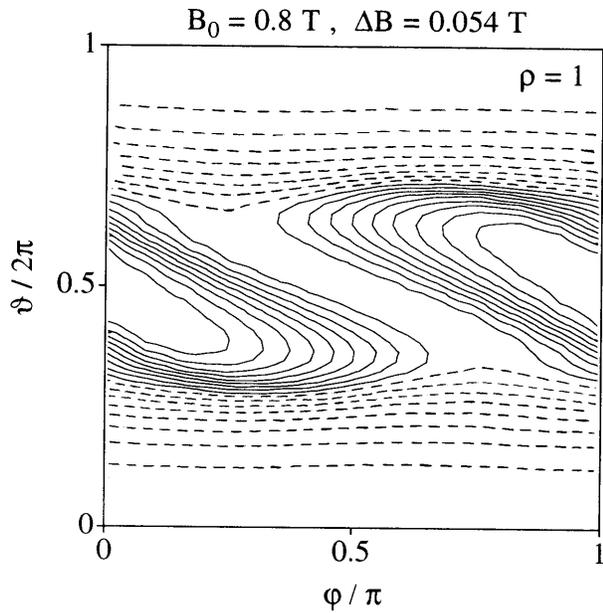
**Fig. 5.**  $|B|$  distribution on the last closed vacuum flux surface of the DHS. Solid contours are for  $B \geq B_0$ , dashed for  $B < B_0$ ;  $\Delta B$  is the difference between adjacent contours.
