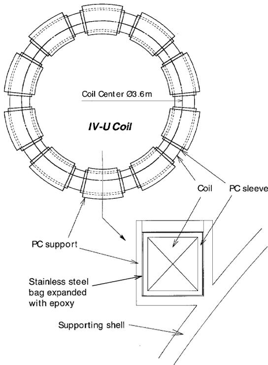
Fig. 1. Top and cross-sectional views of an installed poloidal coil (the upper inner vertical coil).
