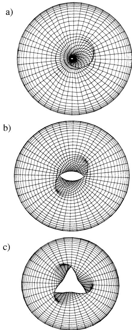
**Fig. 2.** Top view on the last closed vacuum flux surface in (a) SHS, (b) DHS, and (c) THS.
