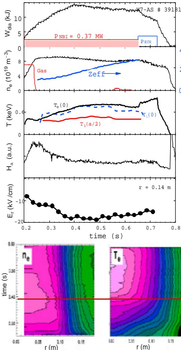
**Fig. 1.** Top part: Time sequences of various experimental quantities during discharge 39181 with maximum  $\tau_E \approx 50$  ms. Bottom part: Density and electron temperature contours of the same discharge. The line indicates the time of energy analysis.
