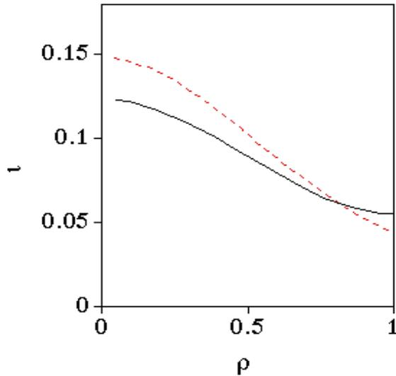
**Fig. 3.** Radial dependence of the rotational transform for the SHS without PF rings (solid curve) and with PF rings (dashed curve).
