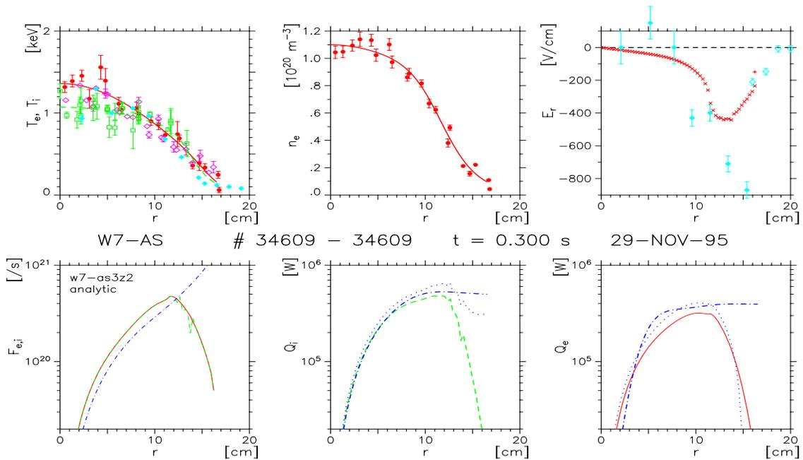
**Fig. 3.** Optimum confinement at high density, discharge 34609, combined ECRH and NBI,  $P_{\text{ECRH}} \approx 350$  kW,  $P_{\text{NBI}}^{\text{abs}} \approx 900$  kW. The symbols are as in Fig. 2.
