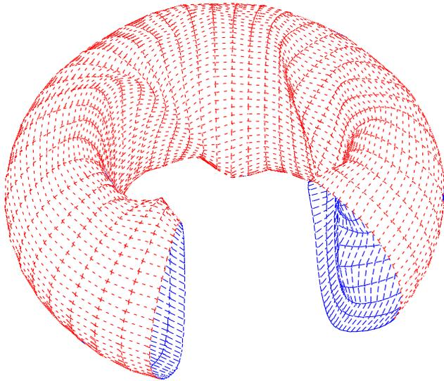
**Fig. 1.** *ksa14\_11*, a 4-period quasisymmetric configuration candidate for NCSX.
