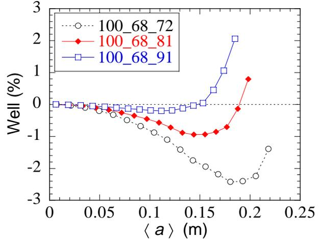
**Fig. 2.** Magnetic well radial profiles for the magnetic configurations investigated in the magnetic well scan experiment.
