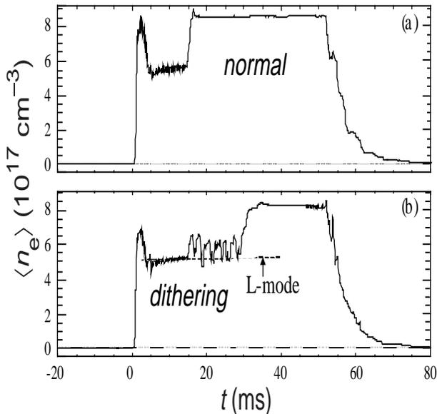
**Fig. 1.** Time traces of the line-average density in H-1 discharges, showing (a) normal and (b) "dithering" transitions to high confinement.
