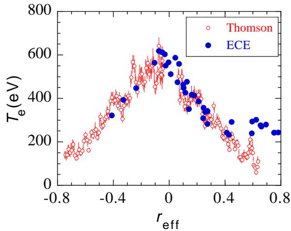
**Fig. 1.** Comparison of electron temperature profiles obtained from second harmonic ECE and Thomson scattering measurements; Thomson data are obtained in a single shot of the discharge series with  $\epsilon(0) \sim 1.51$ . The maximum that appears on the low field side of the ECE profile is due to the presence of a suprathermal electron population.
