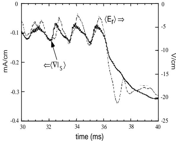
**Fig. 3.** Time traces of electric field and gradient of ion saturation current (measured with a Langmuir probe array) for a discharge with dithering transitions. The quantities are averaged over the radial region  $0.25 < r/a < 1$ .
