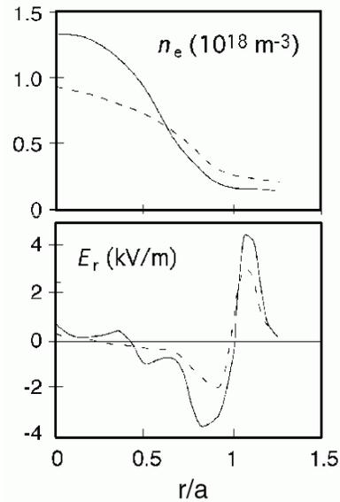
**Fig. 2.** Radial profiles of plasma density  $n_e$  and radial electric field  $E_r$  in H-1. Profiles taken 5 ms before (dotted) and 5 ms after (solid) transition to improved confinement. The plasma boundary  $r/a = 1$  is determined by the last closed magnetic flux surface and is also the location of the helicon wave antenna.
