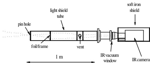
Fig. 1. Drawing of side view of LHD IRVB.
