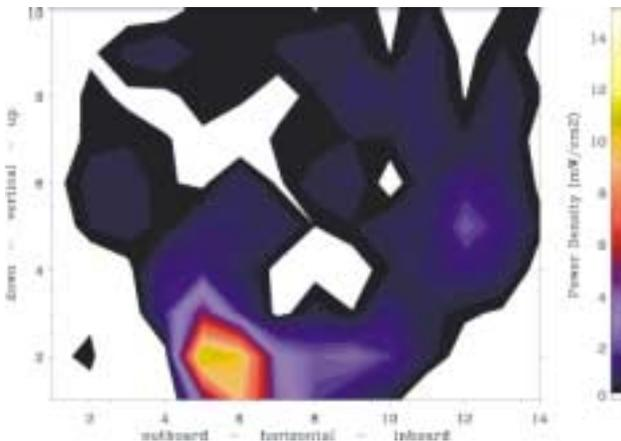
**Fig. 6.** Image from the IRVB during a discharge using an insertable limiter.
