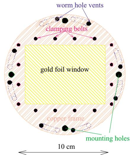
Fig. 2. Drawing of frame for foil of LHD IRVB.
