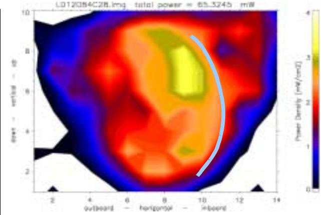
**Fig. 4.** Image from the IRVB during a discharge using the inboard wall as a limiter (blue line shows location of inboard wall).
