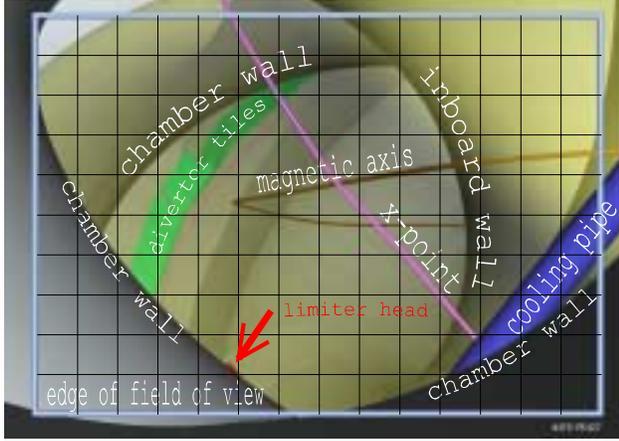
**Fig. 3.** Drawing of the field of view of the LHD IRVB from a tangential port.
