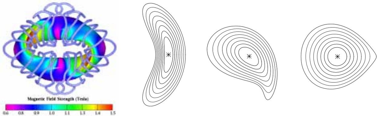
**Fig. 1.** (a) Top view of outer flux surface and modular coils (in blue) for an  $N_{fp} = 2$ ,  $R_0/a = 2.5$  device. (b)–(d) VMEC flux surfaces at toroidal angles  $\zeta/N_{fp} = 0^\circ, 90^\circ$ , and  $180^\circ$ .
