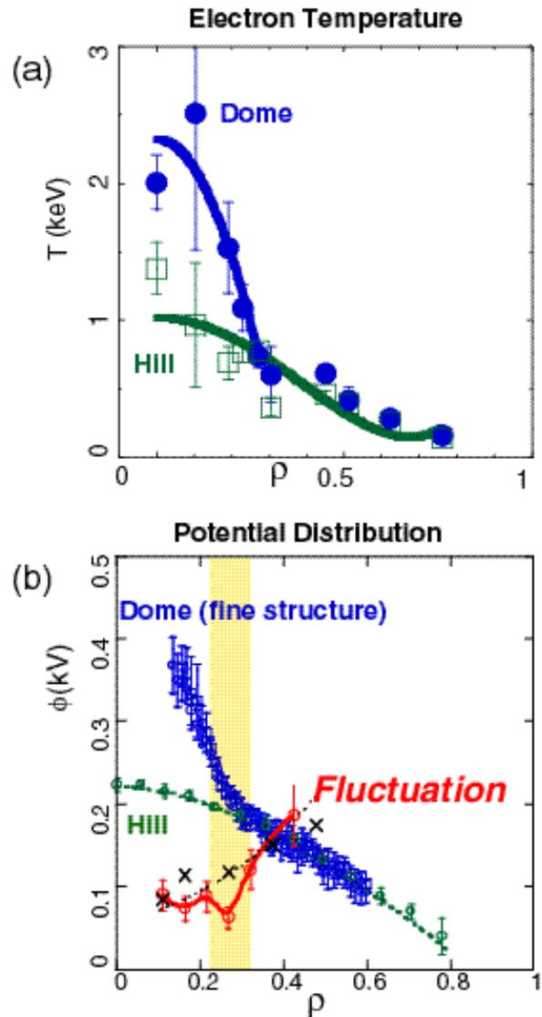
**Fig. 2.** (a) Electron temperature profiles of the dome and hill states. (b) Potential profiles of the dome and hill states, with total fluctuation power of the density. Density fluctuation is reduced where the  $E_r$  shear is maximum.
