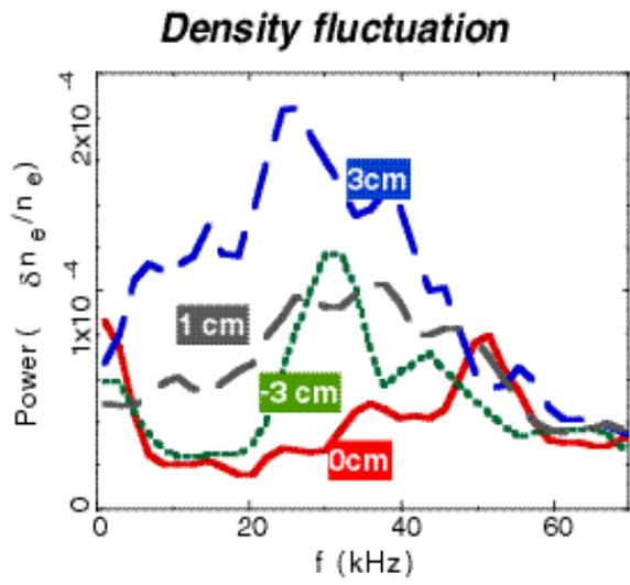
**Fig. 3.** Power spectrum of the density fluctuations around the barrier in the dome state.  $\Delta r = 0$  cm indicates the radius at the transport barrier.
