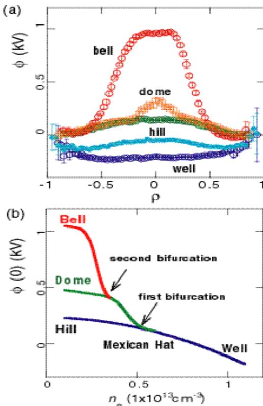
**Fig. 1.** (a) Potential profile patterns in CHS plasmas. All of the potential profiles are observed in ECRH plasmas, while only the *well* shape is identified in neutral beam-heated plasmas. (b) A schematic diagram of central potential as a function of line-averaged density.
