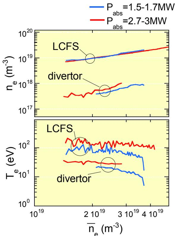
**Fig. 5.** Temperatures and densities at the LCFS and divertor plate are plotted as a function of the average density.
