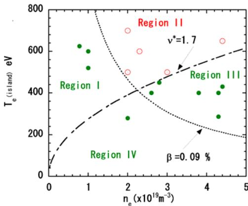
**Fig. 4.** Parameter space ( $T_e(\text{island})$ ,  $n$ ) for island suppression for the case  $w_{ex} = +0.085$ ,  $B = 2.5\text{--}2.75$  T,  $R_{ax} = 3.6$  m. ○ : no island, ● : island with  $w \sim w_{ex}$ . Island suppression occurs in region II.
