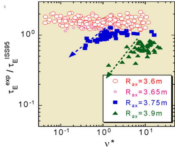
**Fig. 1.** Enhancement factor over ISS95 as a function of  $\nu^*$  for various configurations ( $R_{\text{ax}}$ )
