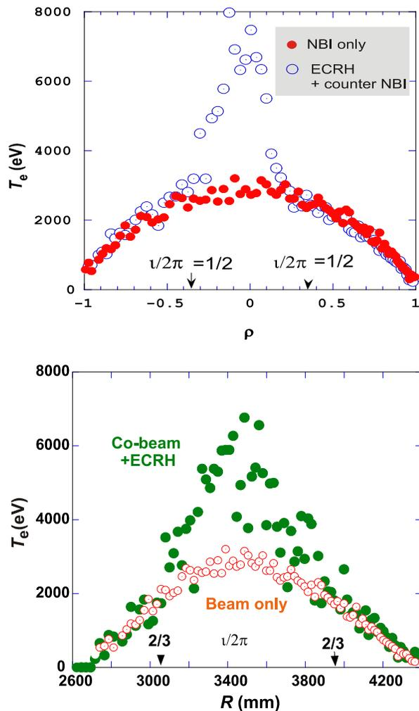
**Fig. 2.** Profiles of  $T_e$  for discharges with NBI only and with NBI and ECRH. The profiles are broad with NBI only, but an ITB forms when ECH is added to both counter- (top) and co-injected (bottom) discharges. In both cases,  $B = 2.84 \text{ T}$ ,  $R_{\text{ax}} = 3.5 \text{ m}$ ,  $n = 6 \times 10^{18} \text{ m}^{-3}$ .
