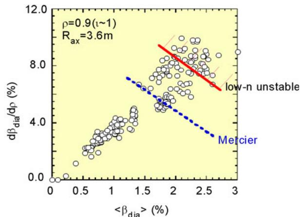
**Fig. 3.** Unstable regimes of edge MHD modes which resonate with  $\nu/(2\pi) = 1$  surface in the parameter space ( $d\beta/d\rho$ ,  $\beta$ ). The observed data points are also shown for comparison.
