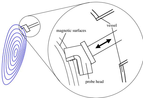
**Fig. 1.** Arrangement of the angular Langmuir probe array on a reciprocating probe drive, depicted together with flux surfaces of W7-AS for rotational transform  $t \approx 0.33$ .
