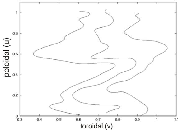
**Fig. 2.** The NCSX modular coils consist of three distinct coil types, shown as a function of the normalized toroidal ( $v$ ) and poloidal ( $u$ ) angles.
