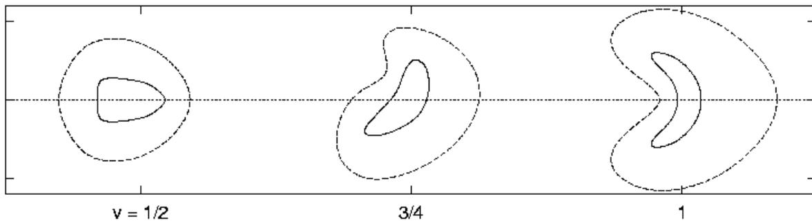
**Fig. 1.** The optimized coil-winding surface shape (dashed line) and reference plasma shape (solid line) shown for three planes in the normalized toroidal angle ( $v$ ).
