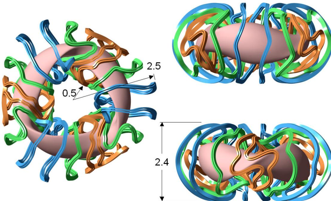
**Fig. 3.** NCSX plasma and modular coils.
