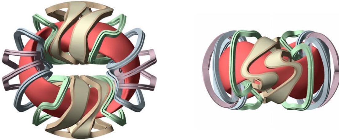
**Fig. 4.** QPS plasma boundary and modular coils for configuration 0718.
