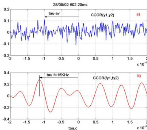
**Fig. 7.** Cross-correlation for (a) non-filtered, and (b) filtered signals ( $f = 15$  kHz).
