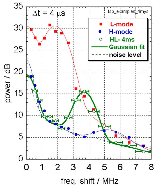
Fig. 1. Doppler reflectometer output at the time of an H- to L-mode back-transition.
