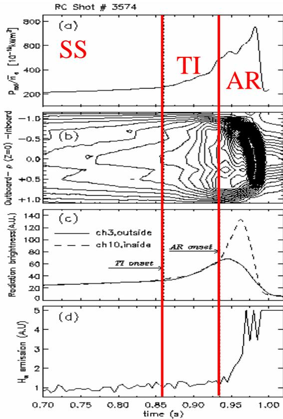
**Fig. 1.** Evolution of radiative collapse in LHD. (a) The ratio of the total radiated power to the line-averaged electron density, (b) radiated power brightness profiles at the vertically elongated plasma cross section, observed at Port 6.5, (c) signals from inboard and outboard bolometer channels of the bolometer at Port 6.5, and (d) the  $H_{\alpha}$  signal.
