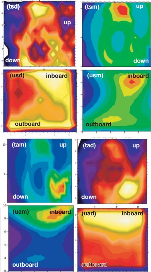
**Fig. 3.** IRVB radiation brightness image data (d) from upper (u) and tangential (t) ports during the steady-state (s) and asymmetric (a) phases of the discharge compared with reconstructions from model (m) profiles.
