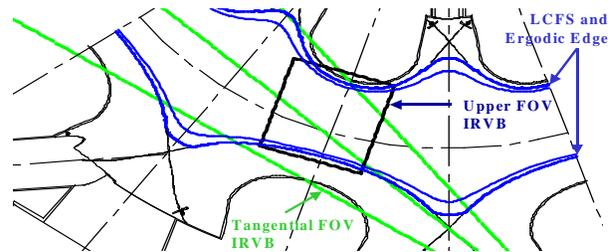
**Fig. 2.** Top view of LHD showing the last closed flux surface (LCFS) and ergodic edge (blue) with fields of view of IRVBs at Port 6.5 (black) and a tangential port (green).
