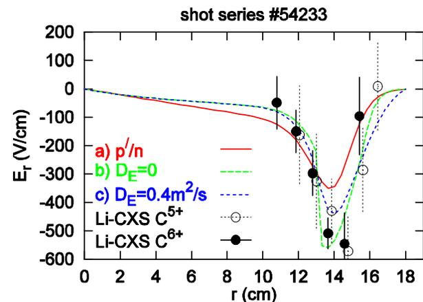
**Fig. 1.** Radial electric field measured by the Li-CXS diagnostic (symbols). The data of  $C^{6+}$  have higher accuracy. Results from neoclassical theory: (a) the approximation proportional to the pressure gradient; (b) the solution of the algebraic ambipolarity constraint; (c) the solution of a diffusion equation for the radial electric field based on a thermodynamic approach. The diffusivity originates from the plasma viscosity.
