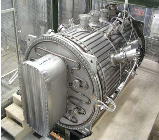
**Fig. 1.** Stray radiation test chamber,  $l = 2.20$  m,  $d = 1.5$  m.
