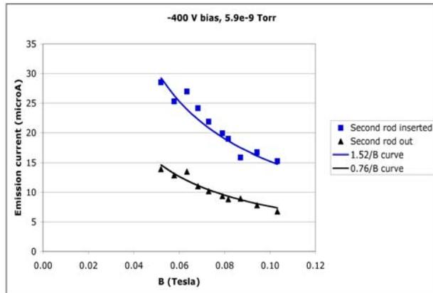
**Fig. 2.** The steady-state emission current as a function of magnetic field strength for two cases — one ceramic rod inserted deep into the magnetic surfaces (black) or two rods inserted (blue). The emission current follows an approximate  $1/B$  scaling and is approximately a factor of two higher when the second rod is inserted, indicating a 50% reduction in confinement time.
