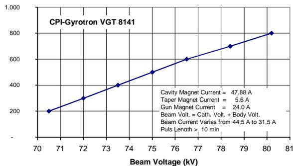
**Fig. 1.** Top: RF power as measured by the calorimeter vs time. Bottom: RF power vs beam voltage (with varying beam current). The measured power is the Gaussian fraction of the gyrotron beam.
