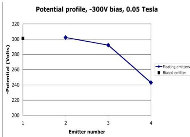
**Fig. 1.** A typical potential profile for a plasma created with a  $-300\text{-V}$  bias on the innermost emitter, which was placed near the magnetic axis. These emitters were spaced approximately  $8\text{ cm}$  apart, with the fourth emitter inside but near the last closed flux surface.
