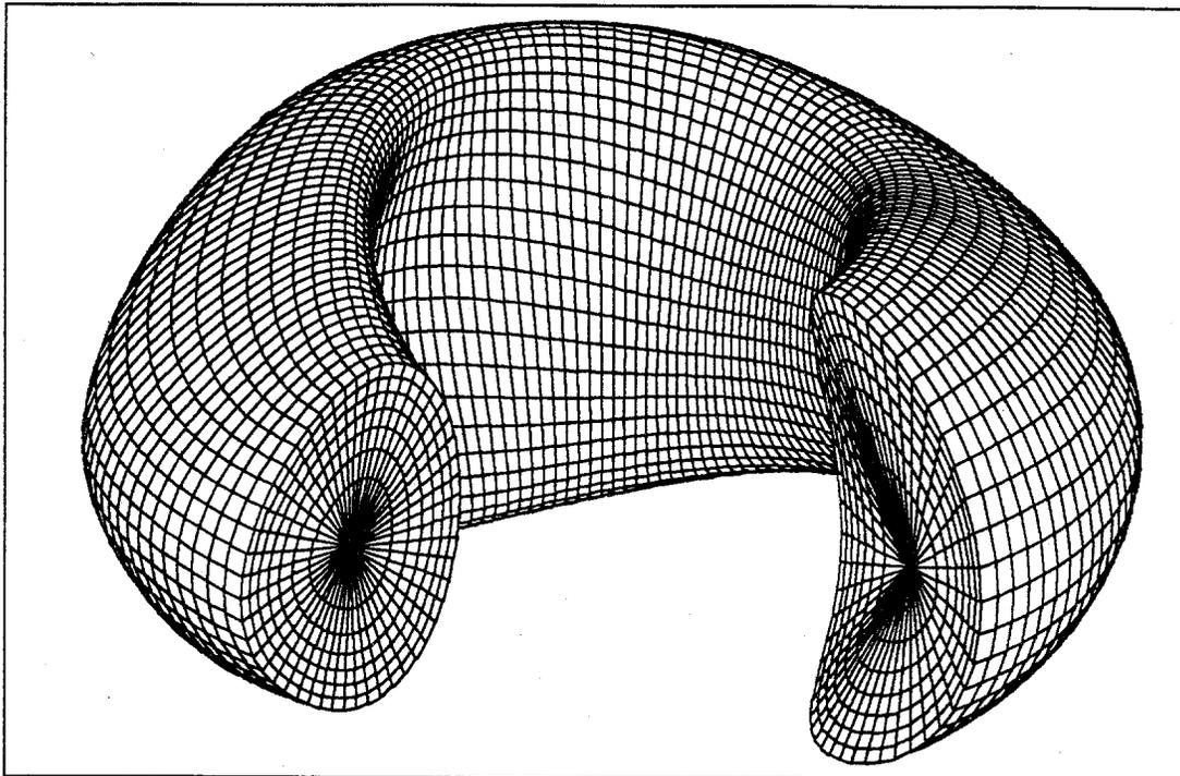
Fig. 5. The LCFS for a quasi-axisymmetric stellarator configuration in which 60% of the rotational transform is produced by the bootstrap current.
