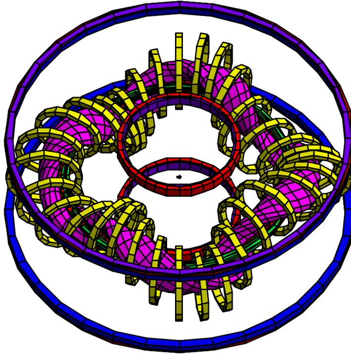
Fig. 4. The coil sets and the last closed flux surface for the TJ-II flexible heliac.
