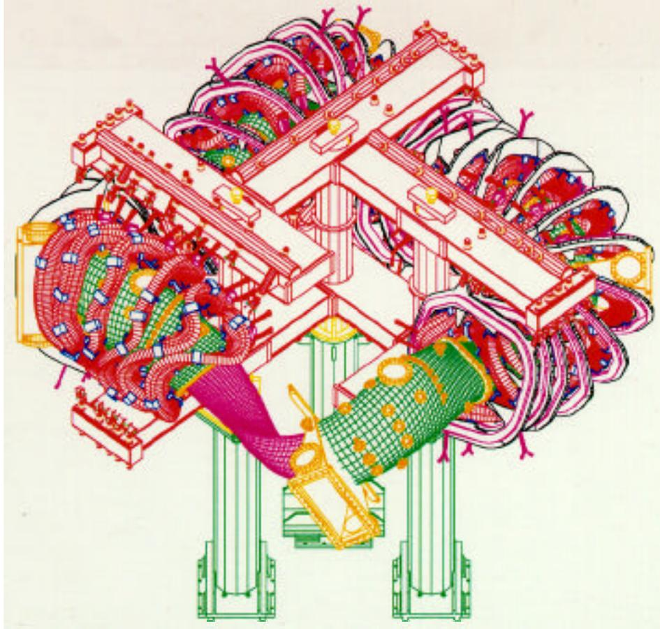
Fig. 8. The LCFS, main nonplanar modular coils, trim toroidal field coils, and the support structure for the HSX experiment.
