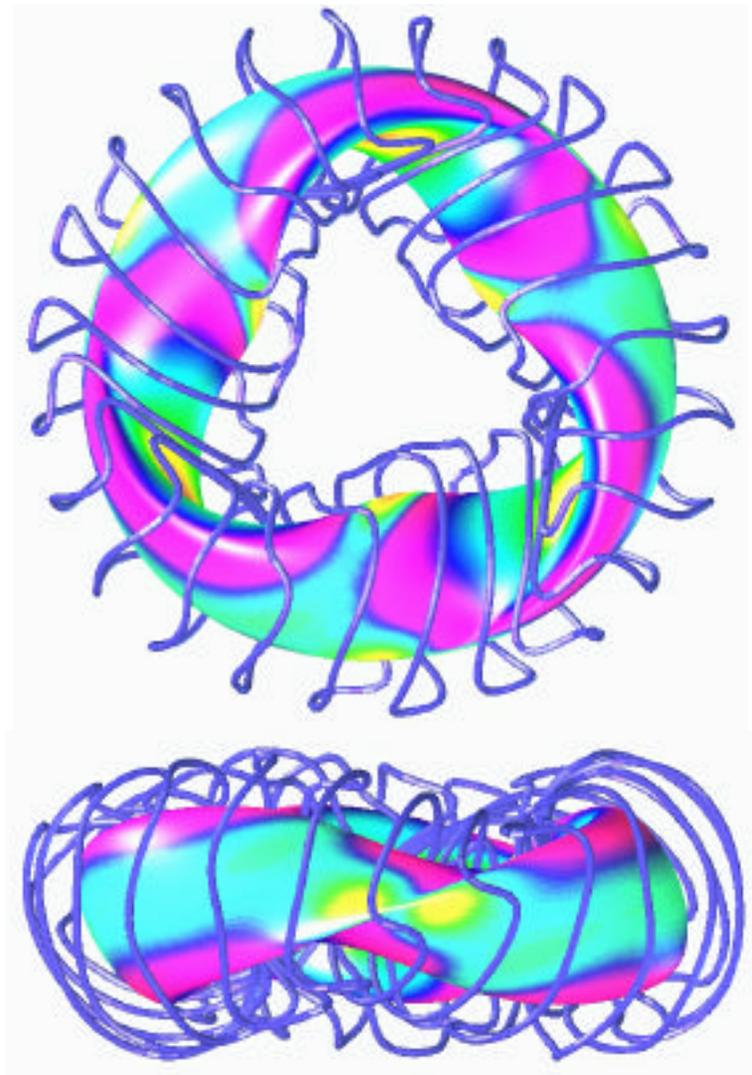
Fig. 6. The LCFS and modular coils for a quasi-omnigenous stellarator configuration in which 10% of the rotational transform is produced by the bootstrap current.
