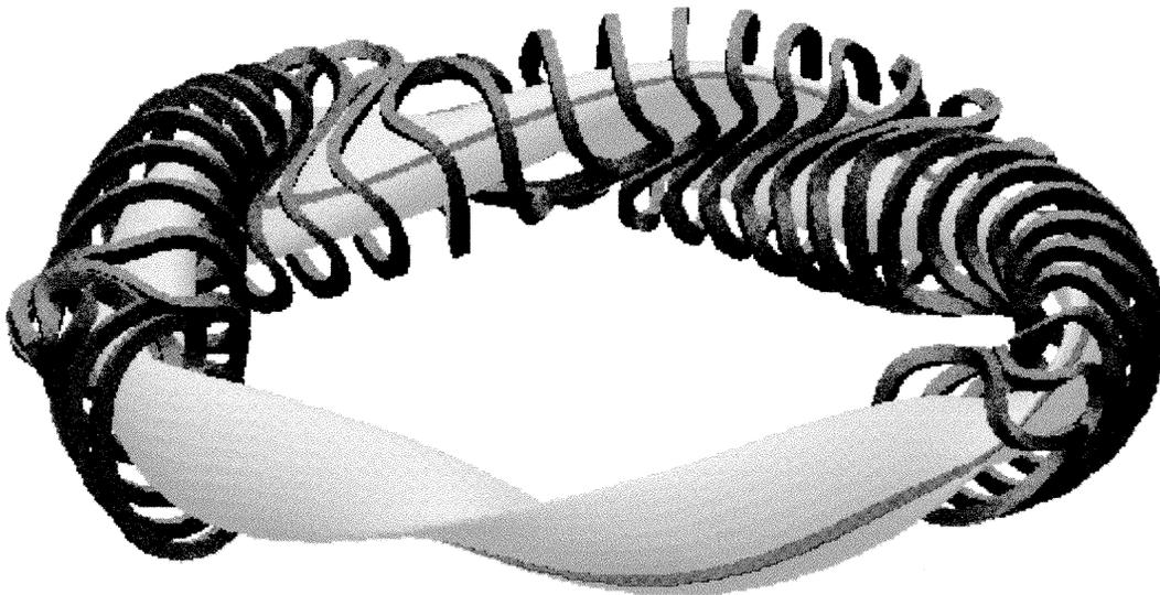
Fig. 3. The modular nonplanar coils and the last closed flux surface for W7-X.
