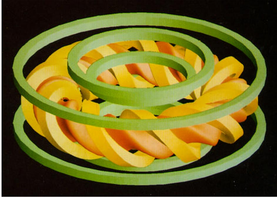
Fig. 2. The last closed flux surface, the helical windings, and the poloidal field coils for LHD.
