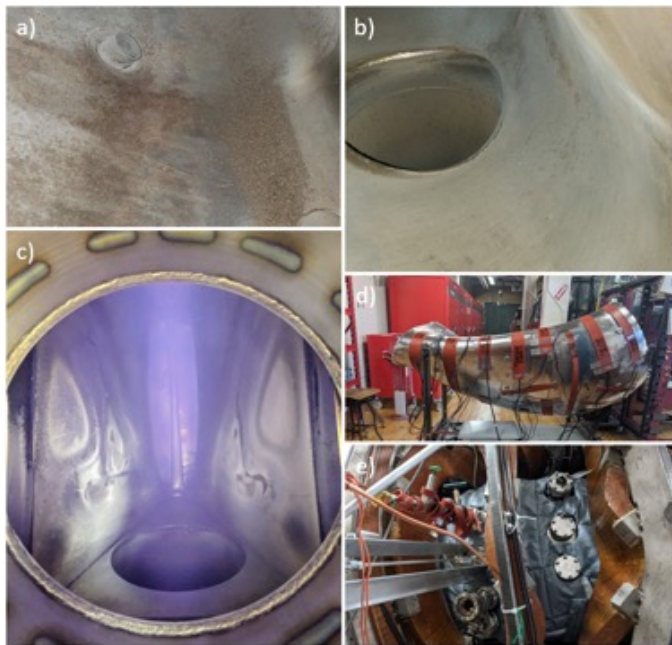
Fig. 1. The inside of the vacuum vessel is seen in (a) before vessel cleaning with significant dust accumulation and (b) after cleaning. (c) Shows an argon glow cleaning discharge in the plasma vessel. (d) A test section of the vacuum vessel with heating tape for the baking system is shown. (e) The grey blanket of the newly installed baking system is shown on HSX.
